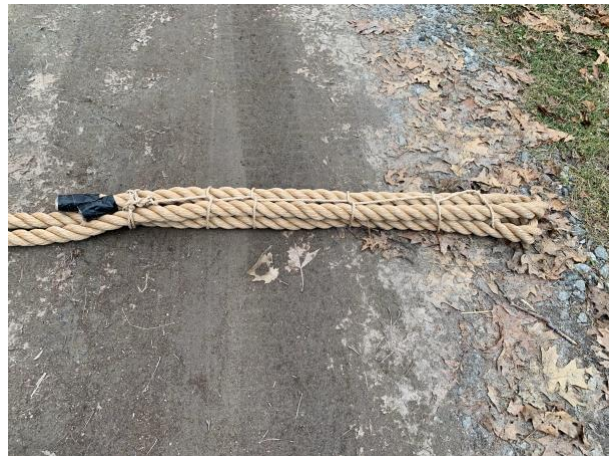
End bundle of a new synthetic speed rope. Note the loop in the cord at the end tie on the far right.
